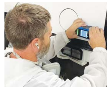
Bryan Thompson captures a picture of a vehicle's finish with the DigiMatch spectrophotometer, which will then be used to create the right formula.
