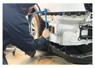
Dillon Turner, a technician at G&C's Berkley facility, uses Glue Pull to straighten a panel.
