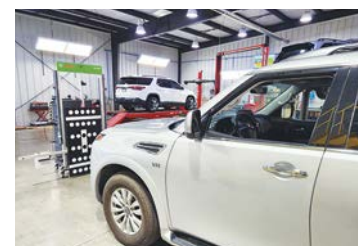
ADAS calibration is set up to be performed on a customer's vehicle.
