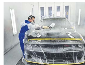
Painter Nery Lopez Barrios shoots clear coat on the hood of a 2020 Dodge Challenger.
