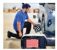
Technician Eduin Garcia of Blue Automotive, Kendrick's specialty division, uses an asTech device paired with the John Bean Tru-Point system to complete static and dynamic calibrations.
