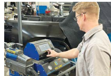
Tyler Stauffer programs and uses Pro Spot's i5 SMART Spot Welder to achieve a high-quality, safe and proper repair. Both Stauffer and Crippen are I-CAR Platinum certified and I-CAR welding certified in all levels.
