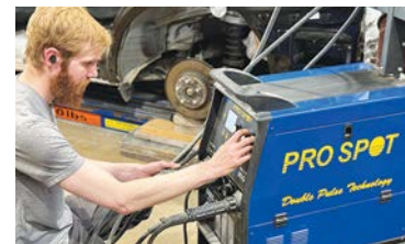
Pro Spot's three-torch SP-5 DP MIG Welder is capable of welding multiple types of metals on a particular vehicle. Technician Alex Crippen is shown programming the welder.
