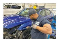
Metro Accident Repair Center technician Gene Taylor uses a KECO Slide Hammer and tabs to avoid intrusive repairs caused by a traditional hammer and dolly technique. DCR partnered with a Toyota dealership in Brook Park, OH, to develop the facility.
