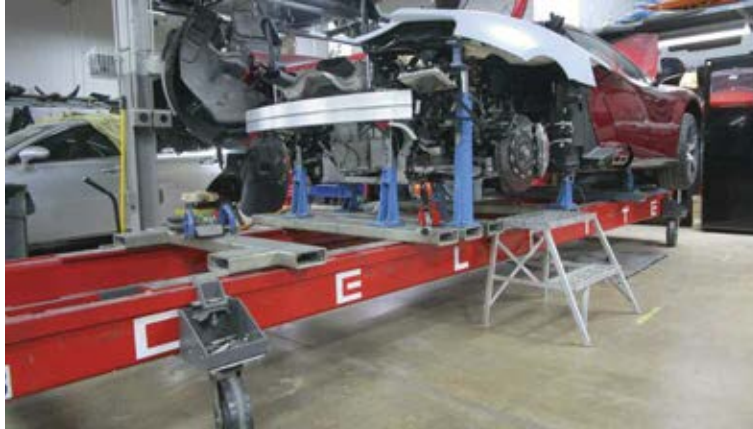
Celette benches have eliminated the guesswork when technicians are doing a repair.
